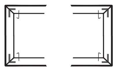
**Step 5:** Roll the screen on the frame. Arrange the sliding hooks so that they are in line with the holes on the screen.
