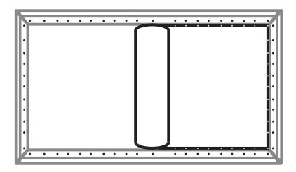
**Step 6:** Tie the fasteners to all the eyelets on the screen. Fasten the fasteners to the sliding hooks on the frame. Fasten all the hooks properly so that there are no wrinkles on the screen. Make sure to fasten 2 fasteners to the hooks on all the four corners of the screen.
